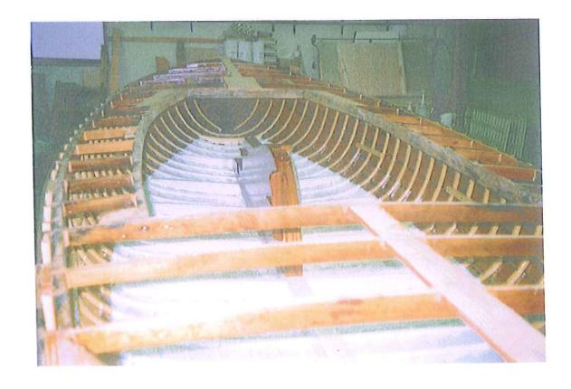
15. Plane in the deckframe fair and fix the decks, fore decks and L shaped aft decks first with scarphs cut. Then lay in sidedecks. Fix the washboards, cockpit bevels and trim, mooring cleat, boom crutch socket, and boom crutch. Fill and fair the topstrakes and fit the gunnel beadings. (Pre-scarph a piece to make both beadings and then rip, bevel and shape the undersides – shape the top outer nosing after fitting).
